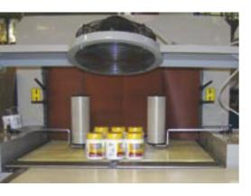
to 10 work programmes and ensures a simple and accurate control of all parameters and production phases, such as: temperature and seal time; opening of seal bar; speed and positioning of pusher; oven temperature; speed of oven belt; etc....
